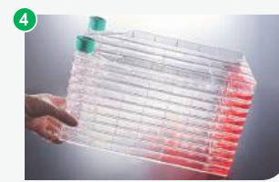
Carefully tilt the Cell Factory system to a horizontal incubation position with the filling inlet up
