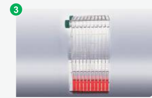
Turn 90° so the filling inlet is in an upward position. The medium will be separated, with equal amounts in each chamber.
