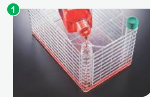
Pour the media directly into the Cell Factory system
